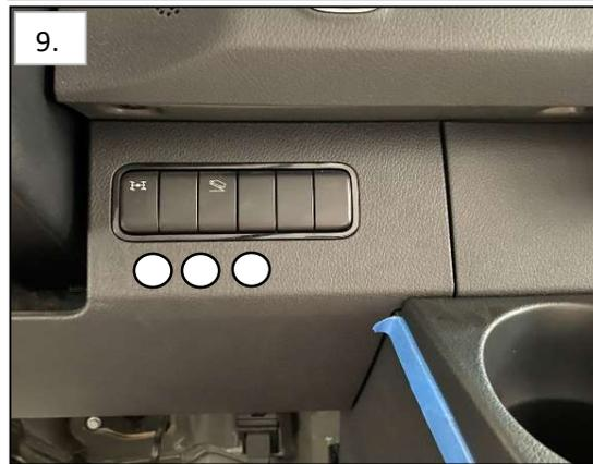
10. If an OEM look is desired, locate an OEM dash switch to replace any of the blank switch covers. Agile Off-Road carries these switches. Ensure the OEM switch is pinned correctly, remove the toggle switch on the supplied Baja Designs harness & hook up to the OEM terminals. The terminals on the Baja Designs harness are as shown.
