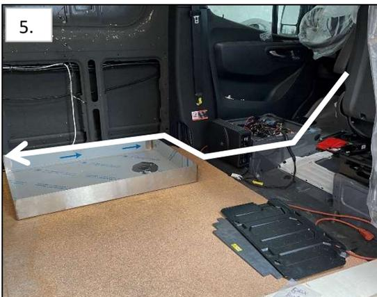
**6.** Use the 3x 10' extension harness where needed to reach the back of the vehicle.
